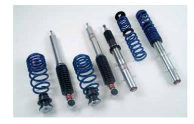
Example of a complete coilover suspension set including component certification:
